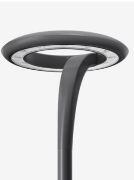
EX1 Manufacturer: DW Windsor Product: Sephora Halo Output: 41.5W, 6330lm Optic: A1, wide road optic Colour Temperature: 3000K Mounting Type: Column Mounting Height: 6m
