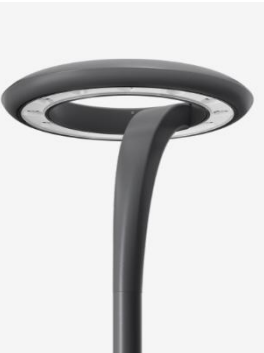
EX2 Manufacturer: DW Windsor Product: Sephora Halo Output: 97.9W, 14630lm Optic: C3, area optic Colour Temperature: 3000K Mounting Type: Column Mounting Height: 6m
