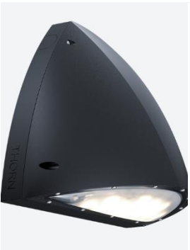
EX5 Manufacturer: Thorn Product: Piazza 3 Output: 13W, 1652lm Optic: Asymmetric Colour Temperature: 3000K Mounting Type: Surface wall Mounting Height: 2.5m To be supplied with integral emergency battery as required for use as an emergency luminaire
