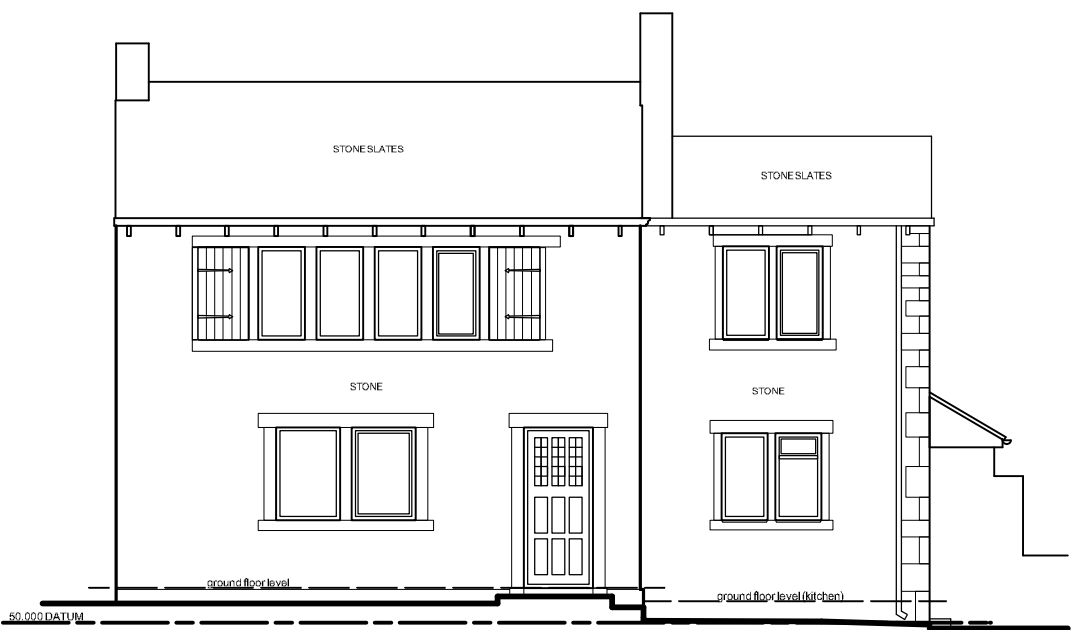
east elevation (as exg)
