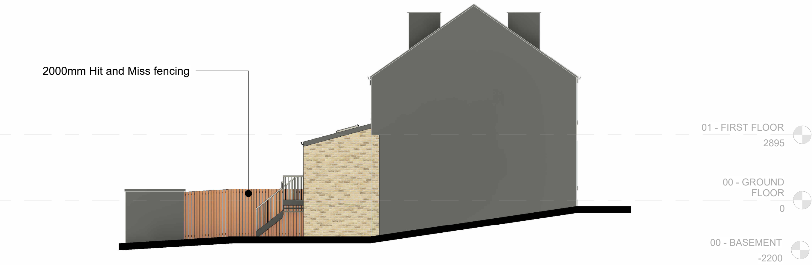
B - NORTH-WEST ELEVATION SIDE 1 1 : 100
