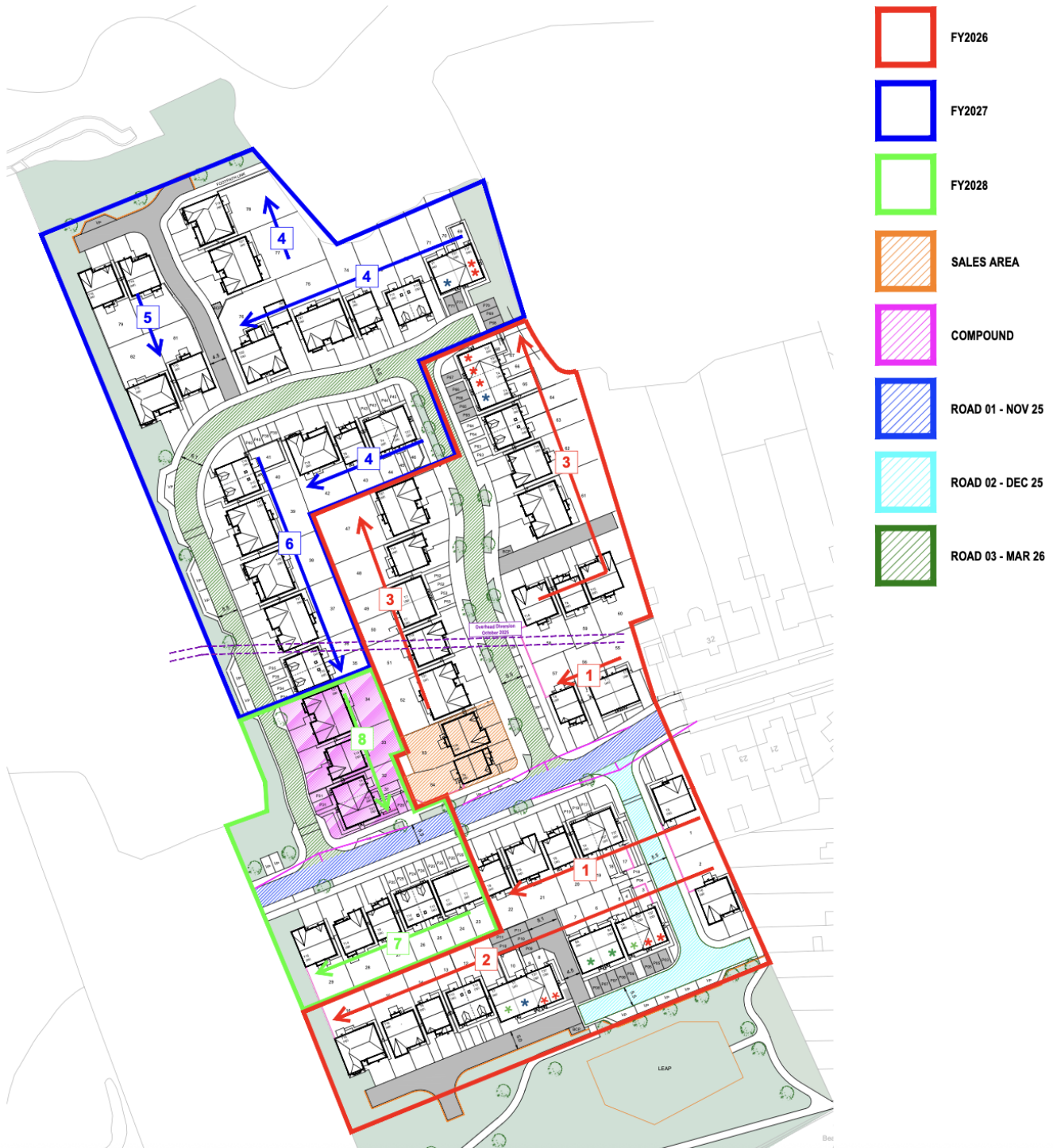
Fig 1. Road phasing, housing phases.
