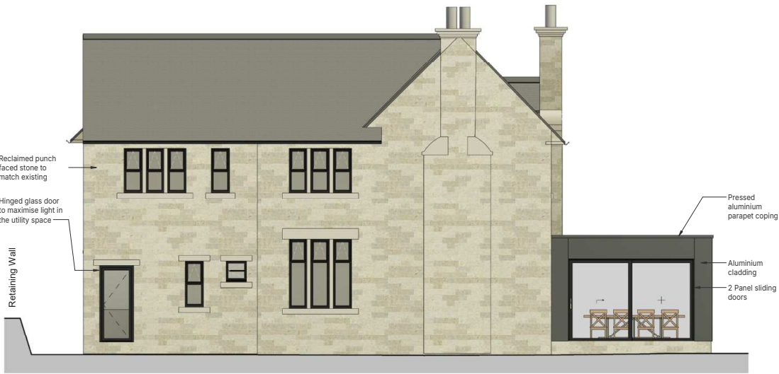
West Elevation - C 1 : 50
