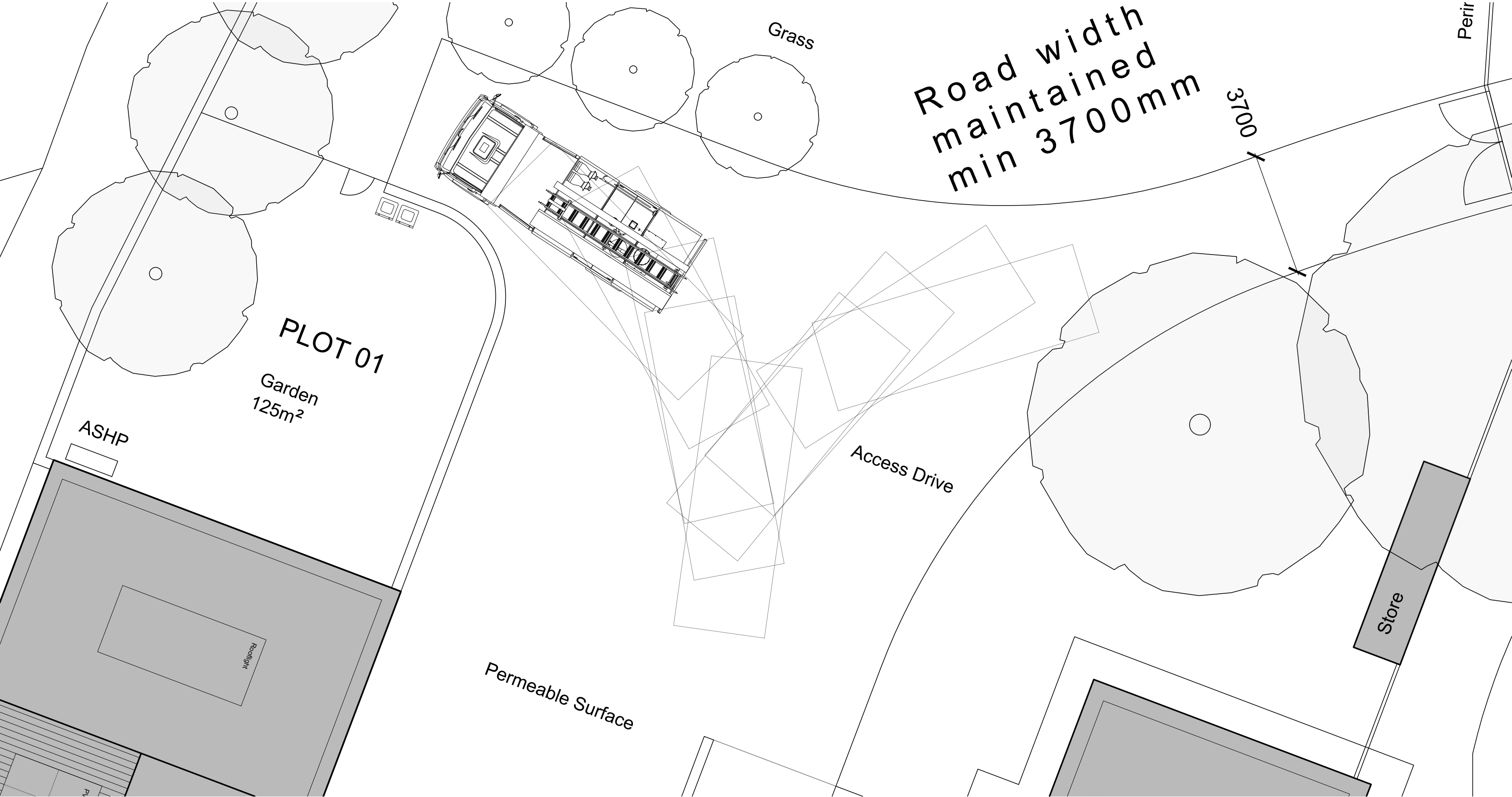
FIRE APPLIANCE TURNING 1:100 @ A1
