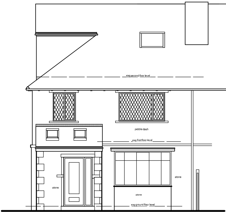
east elevation (as exg)
