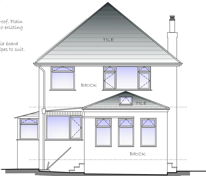
EXISTING REAR (NORTH-EAST) ELEVATION SCALE - 1:100
