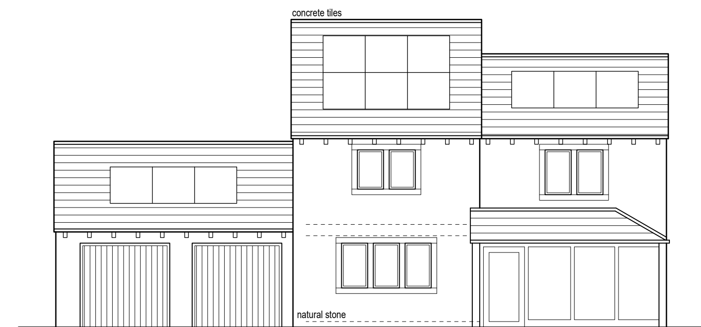
Front/south east facing elevation (1:100)
