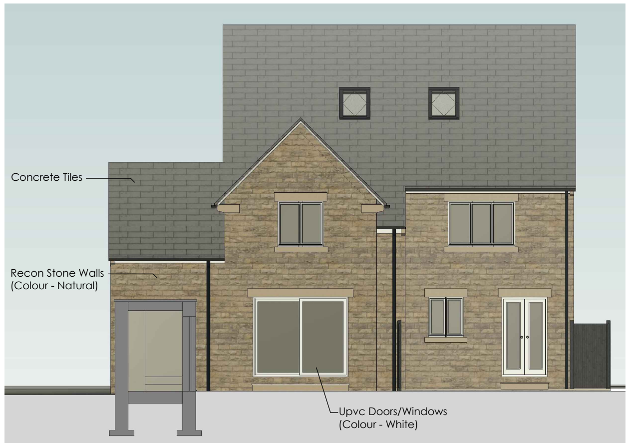
REAR (NE) ELEVATION/SECTION
