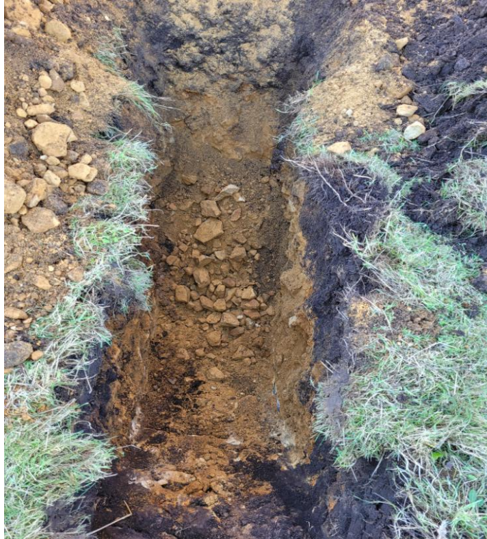
Typical trial pit
