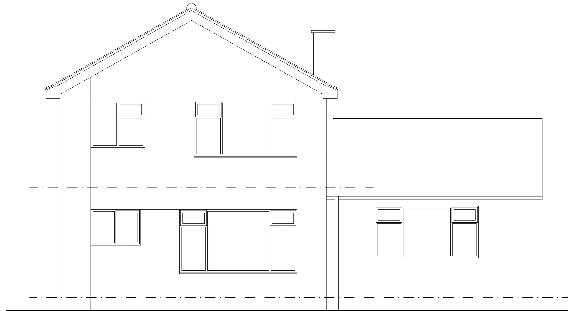
EXISTING NORTH ELEVATION
