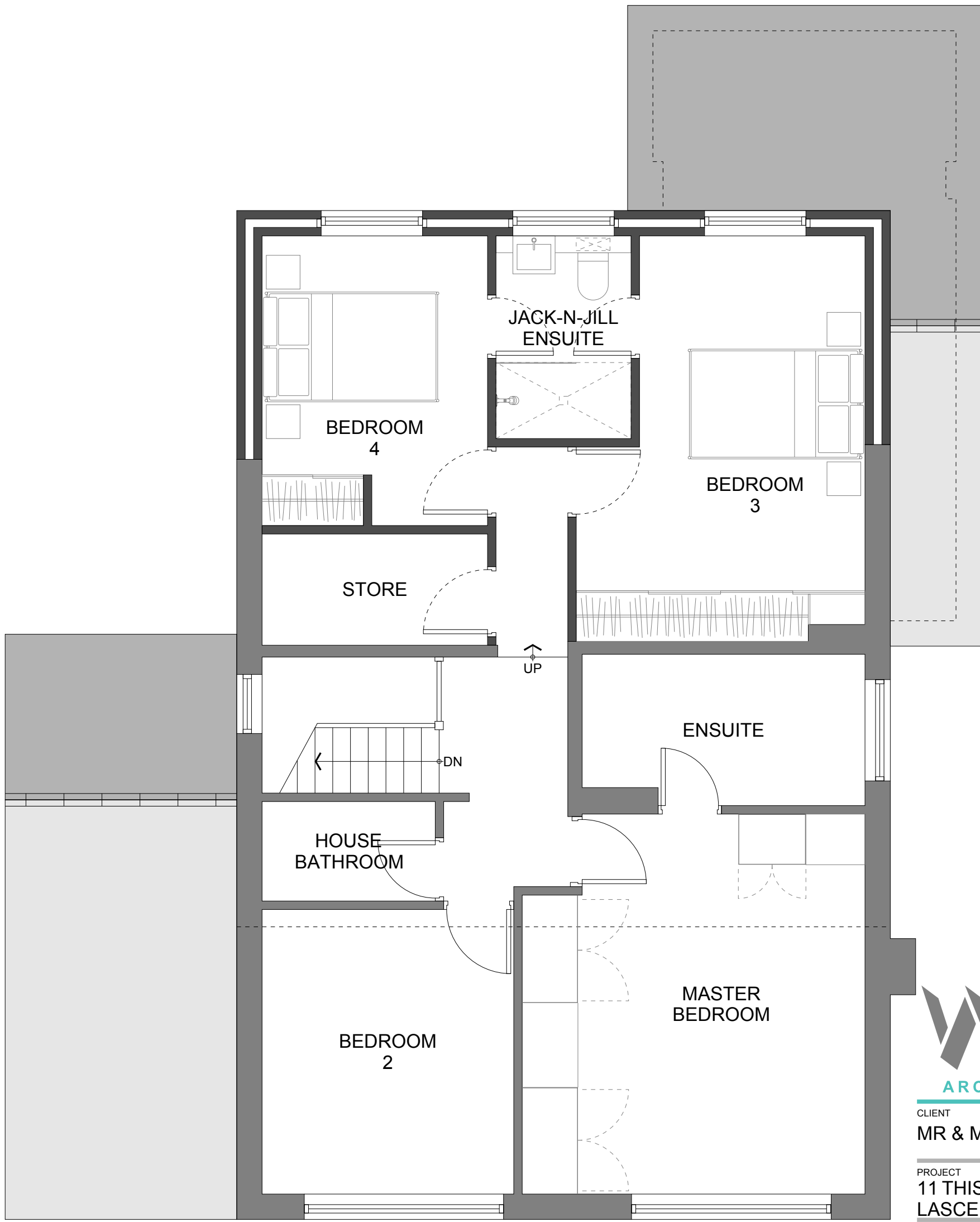
FIRST FLOOR PLAN - 1:50 PROPOSED
