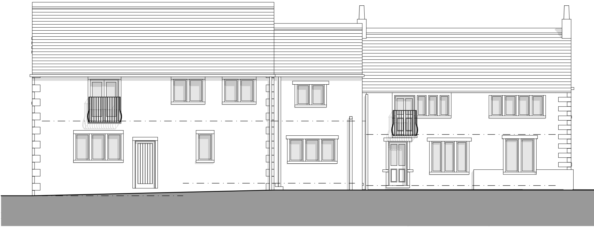
Existing South Elevation - 1:100
