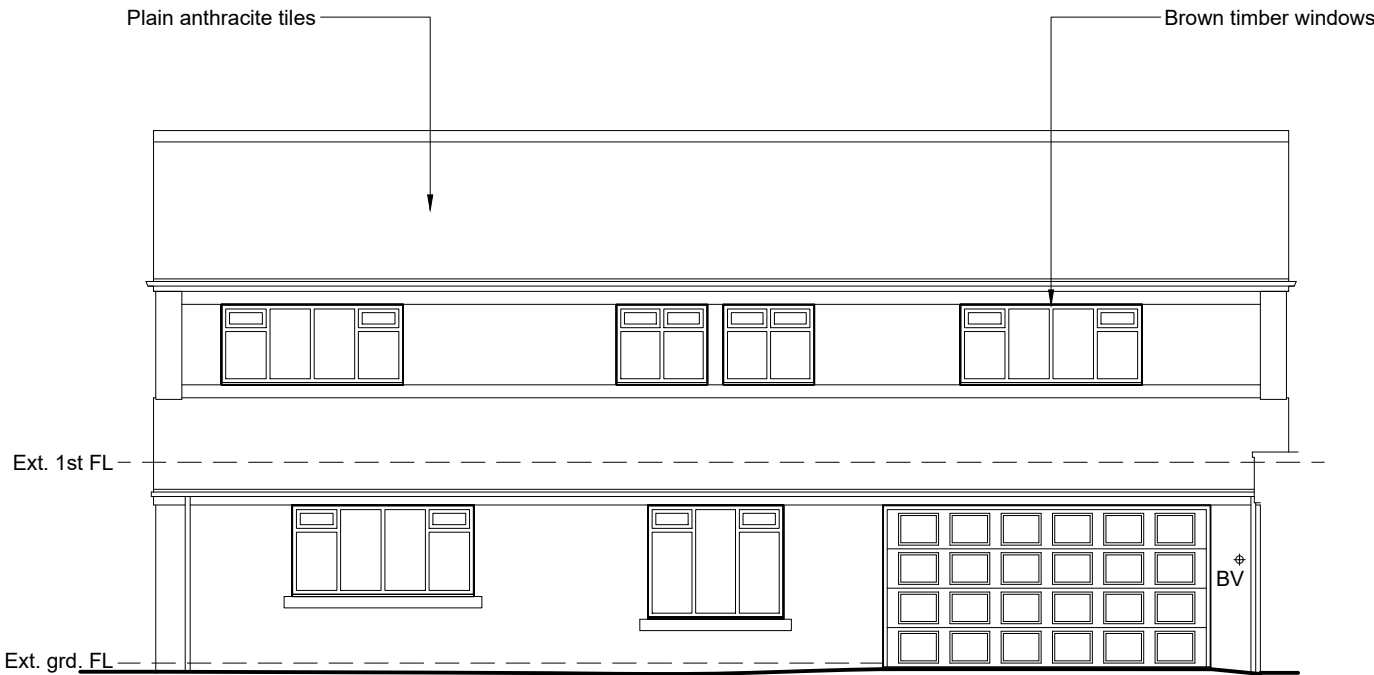
EXISTING PART REAR ELEVATION (C)
