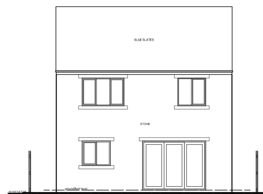
east elevation (as existing)
