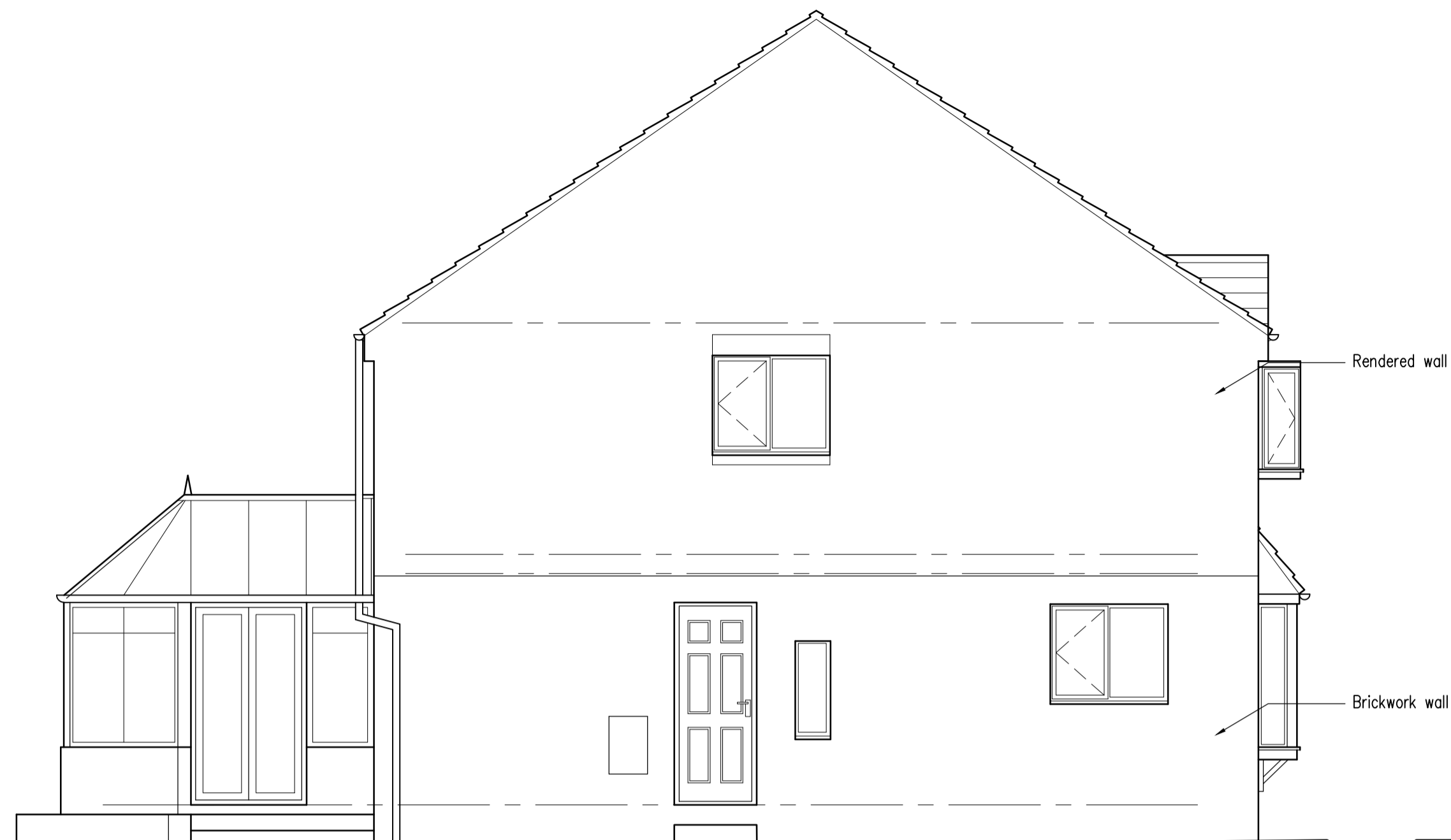
EXISTING SIDE ELEVATION
