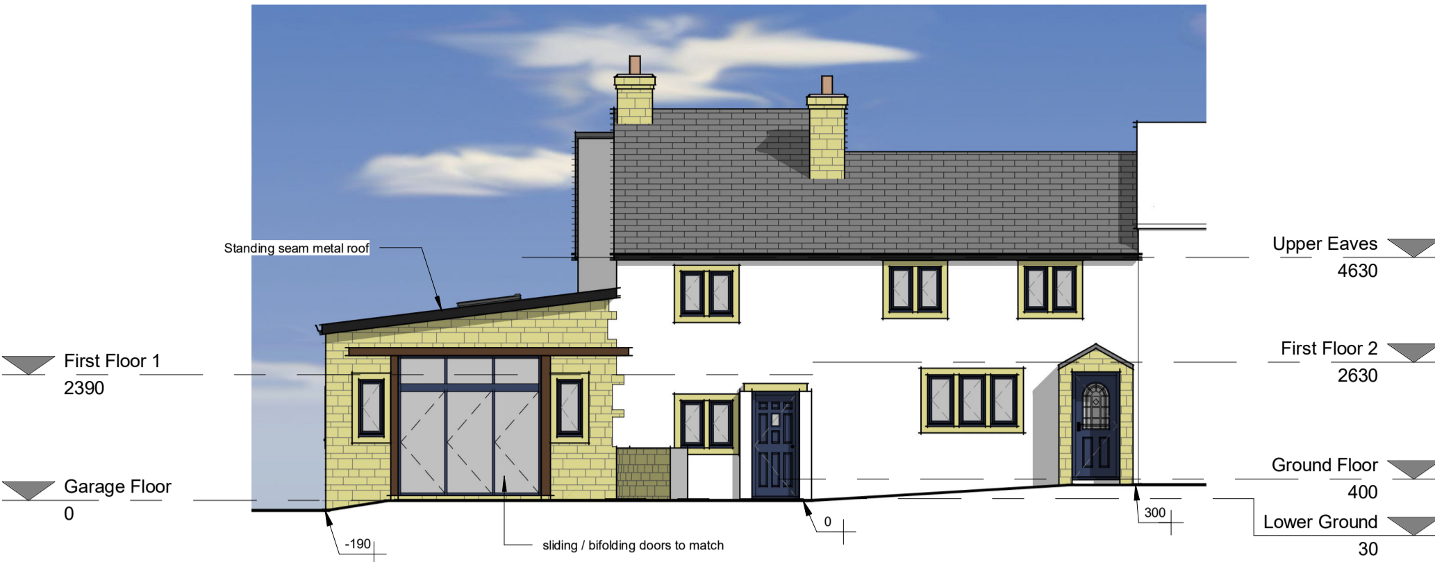
Front Elevation (NW Facing) 1 : 100
