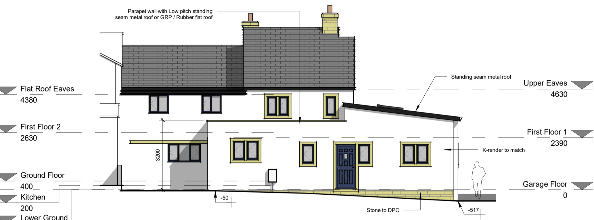
Rear Elevation (SE Facing) 1 : 100
