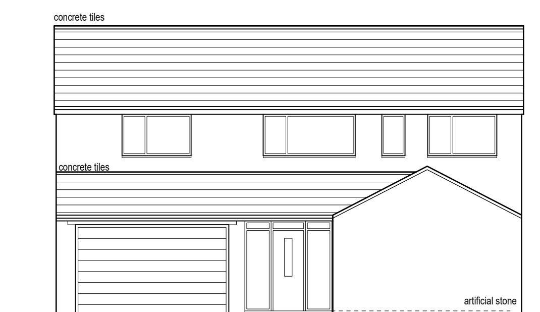
Proposed front/west facing elevation (1:100)
