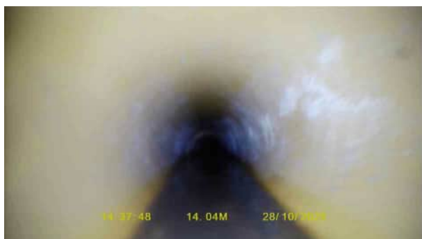
SW5X_db62401e-328e-4946-b53c-390c227c1f6d_20251113_090617_144.jpg, 00:01:29, 14.40 m Water level, 30% of the vertical dimension
