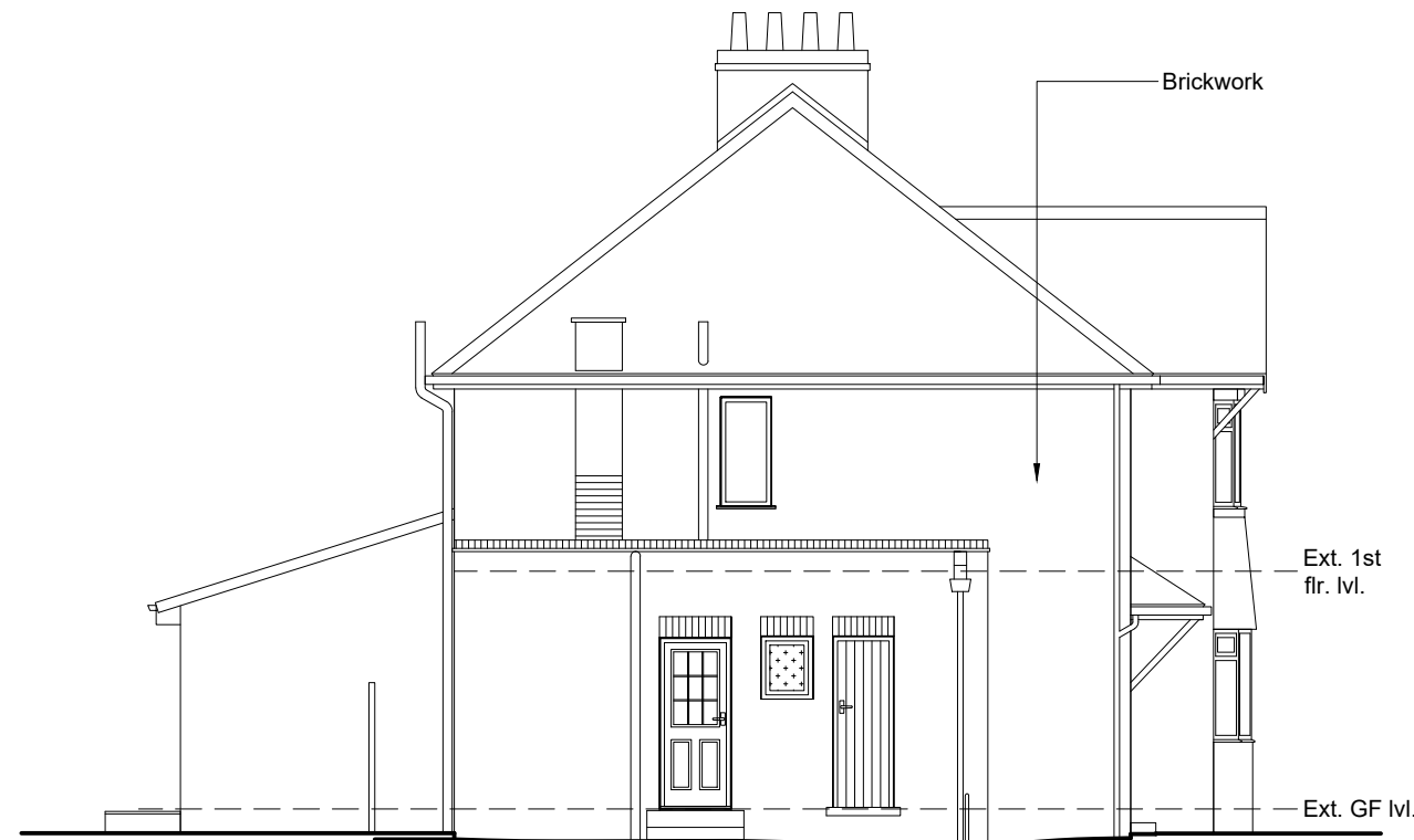
EXISTING SIDE ELEVATION
