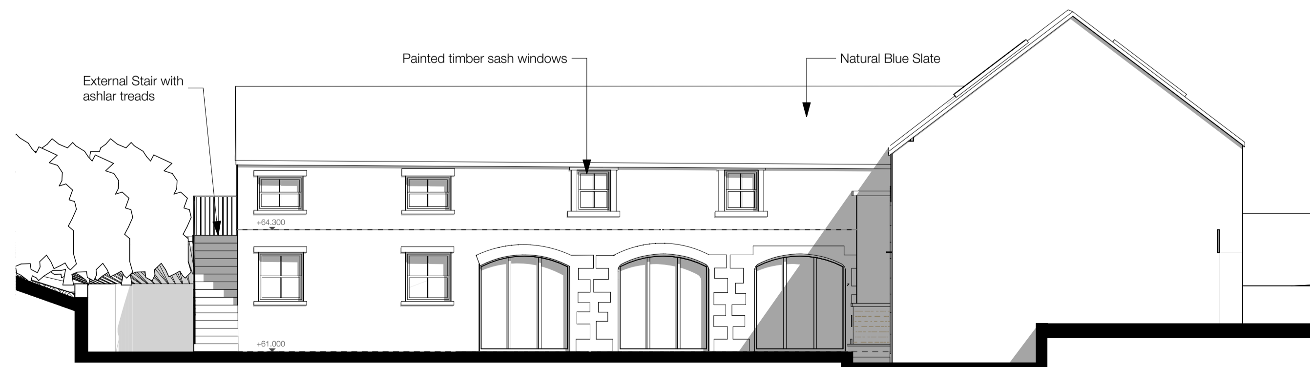
Listed Building East Elevation - 1:100
