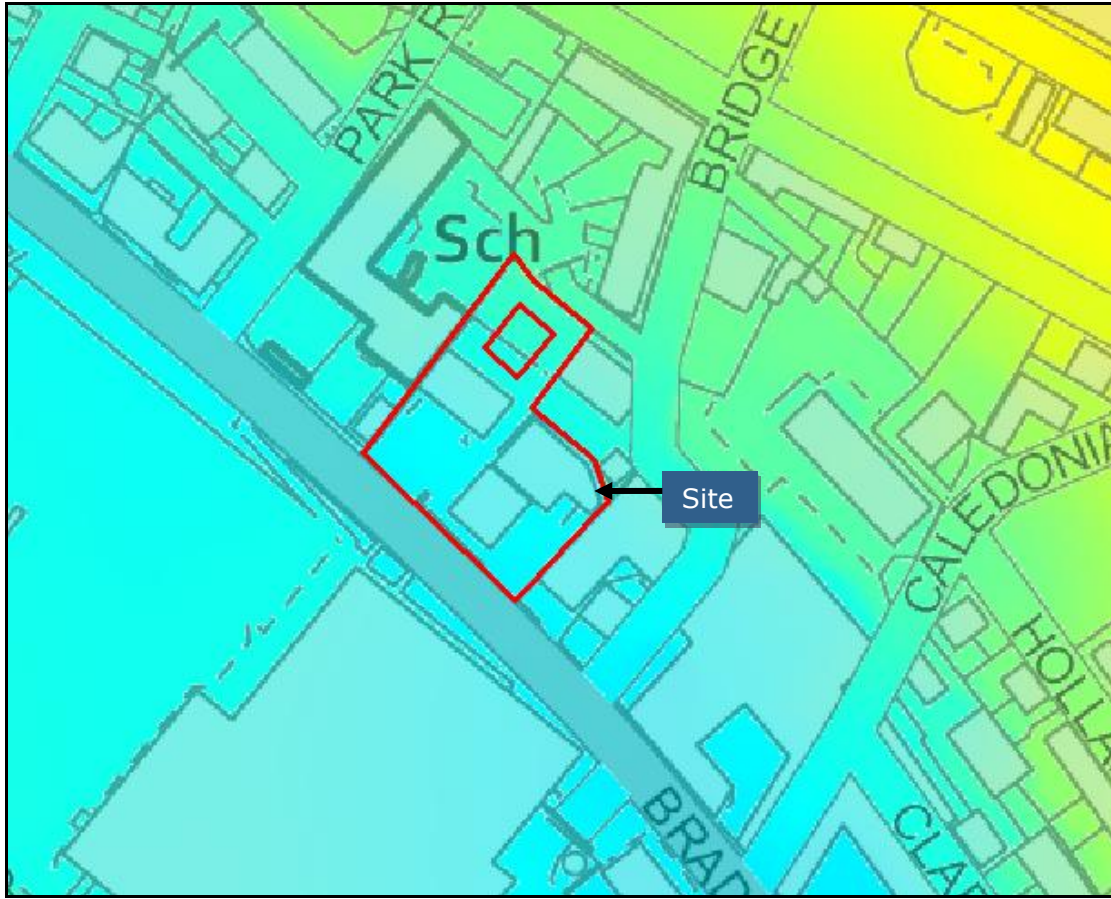
Figure 2: LIDAR survey data where higher ground is denoted as orange and yellow colours and lower areas denoted by blue and green colours
