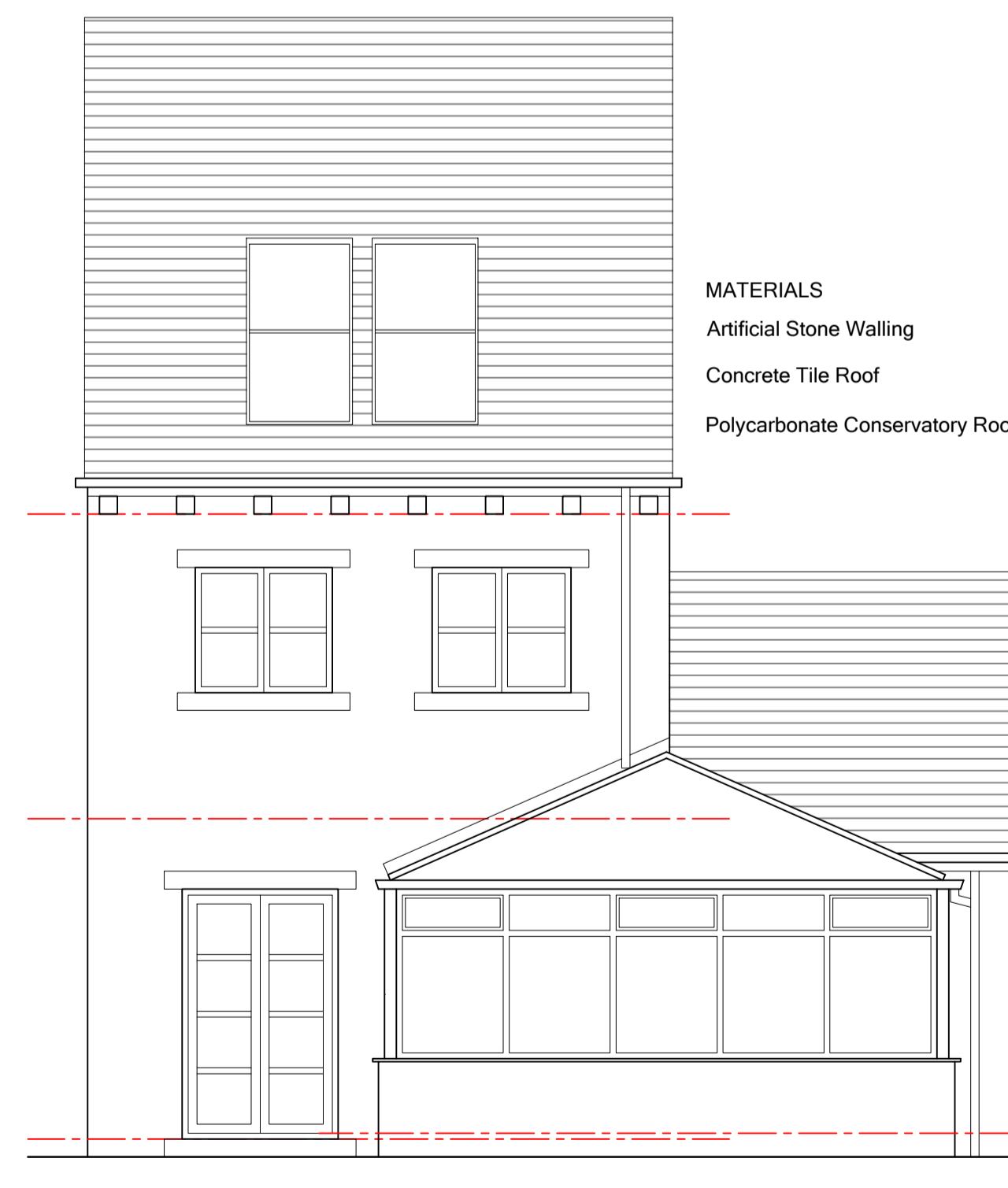
EXISTING NORTH ELEVATION 1:50
