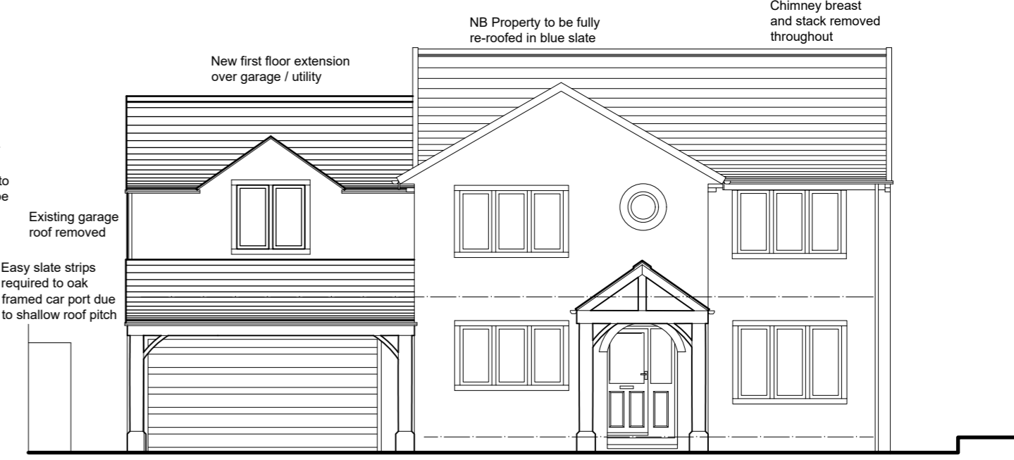
North East Elevation (front)
