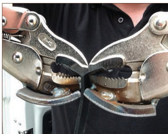
Figure A4.46 Testing a weld with 'dog bone' grips (courtesy MEC Environmental Ltd)
