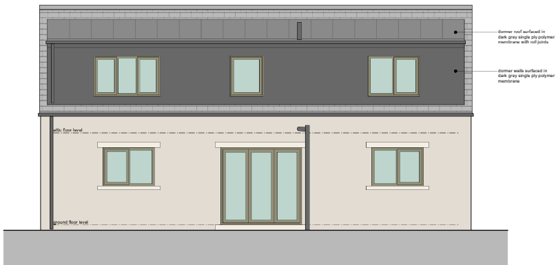
north elevation - rear
