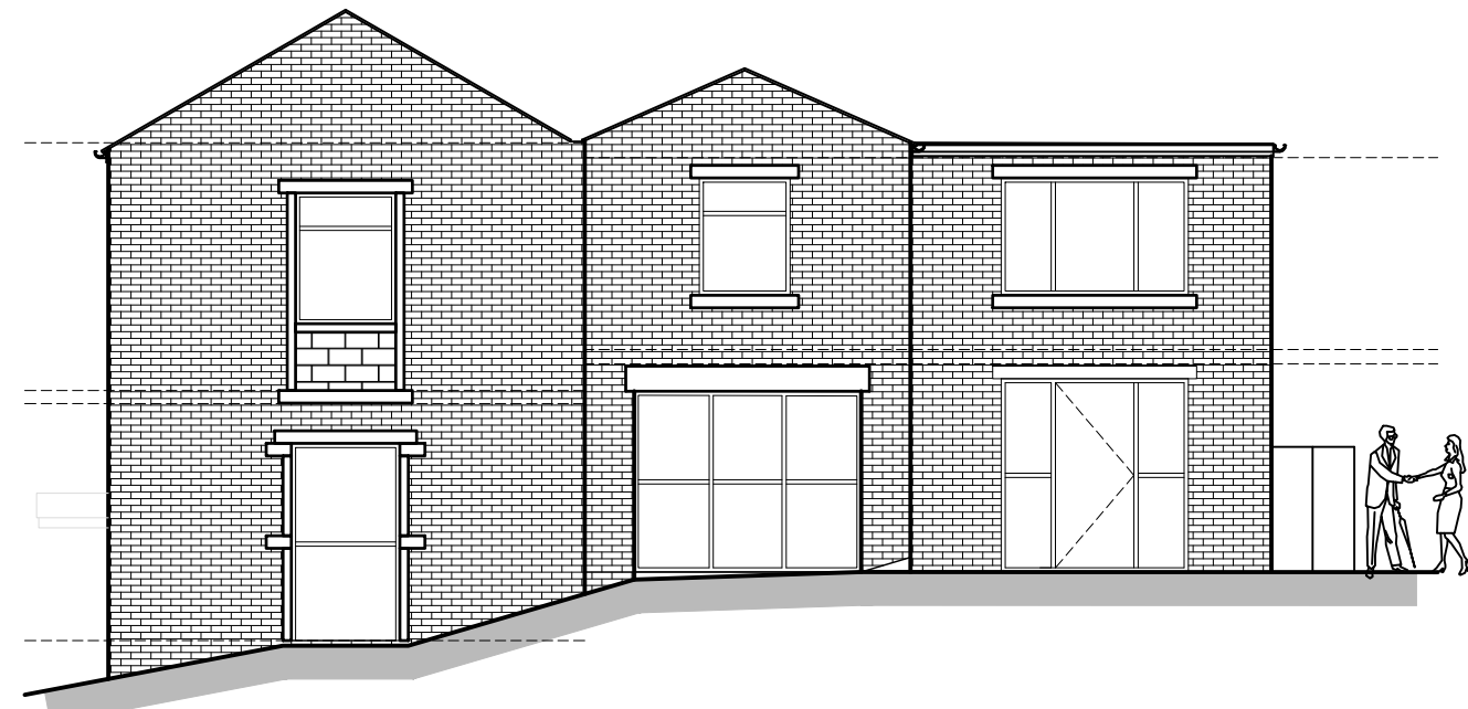
(PROPOSED)(SOUTH EAST) BRIDGE STREET ELEVATION, 1: 100mm
