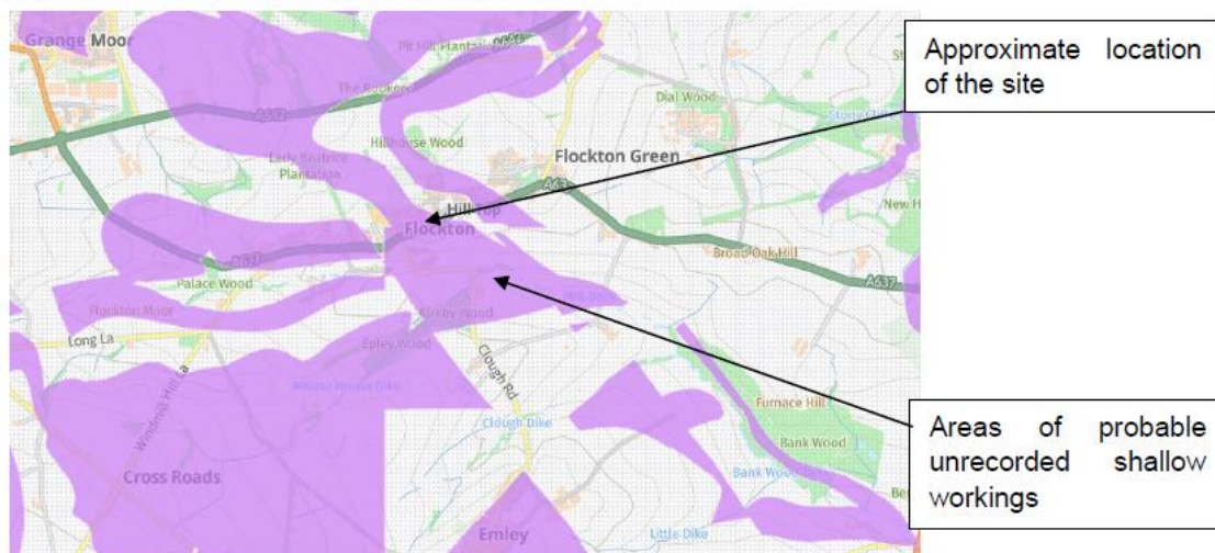
Figure 4.5: Probable Unrecorded Shallow Workings
