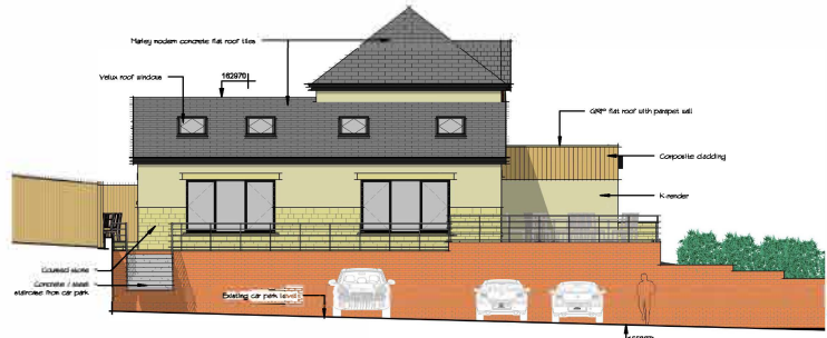
Side Elevation (West Facing) 1 : 100
