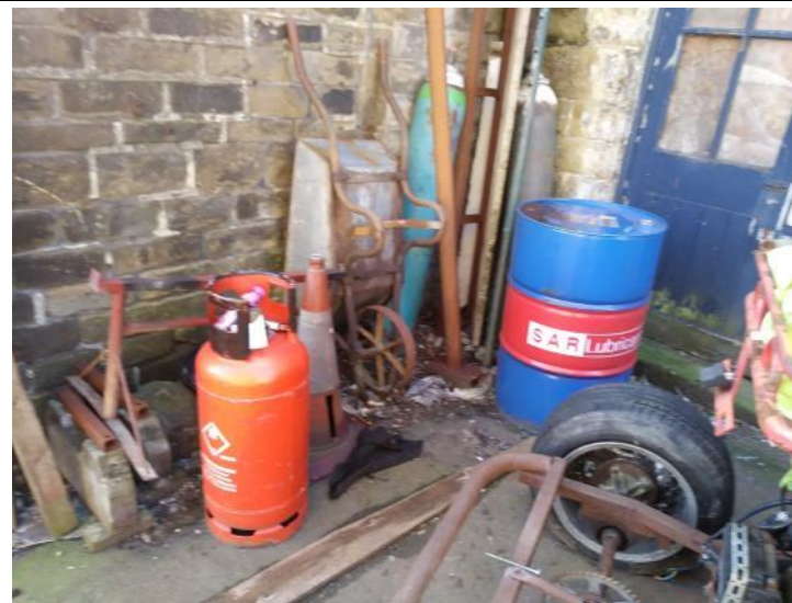
Photograph 58 – Unbundled lubricant barrel and surface oil staining
