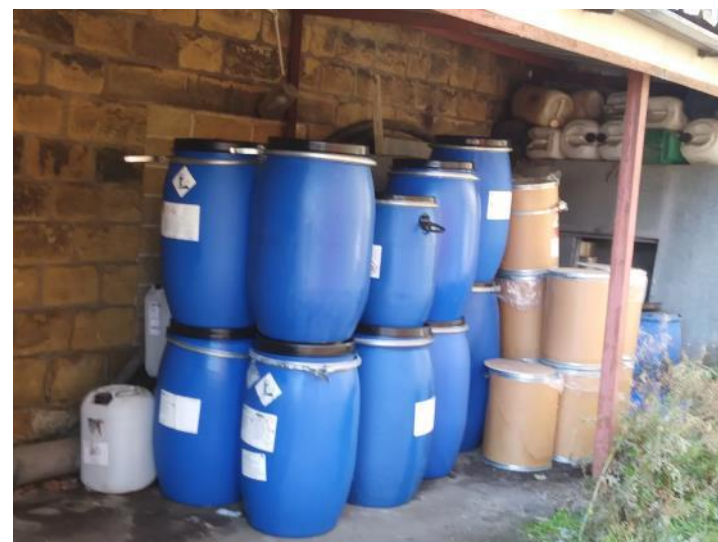
Photograph 48 – Unbunded storage of chemicals
