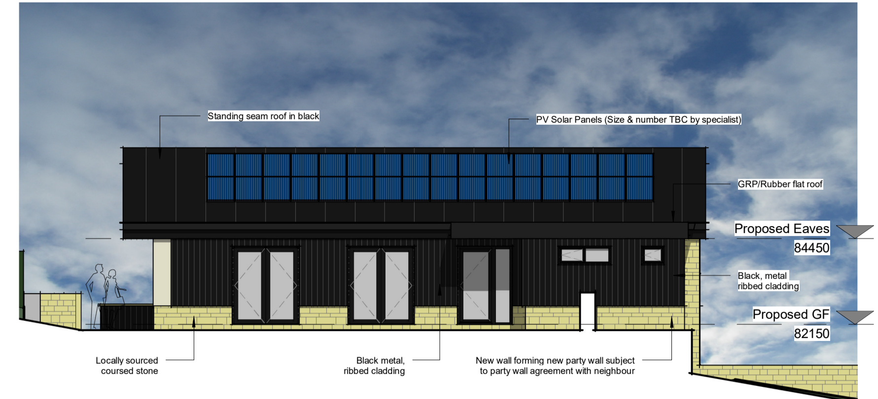
Front Elevation (South Facing) 1 : 100
