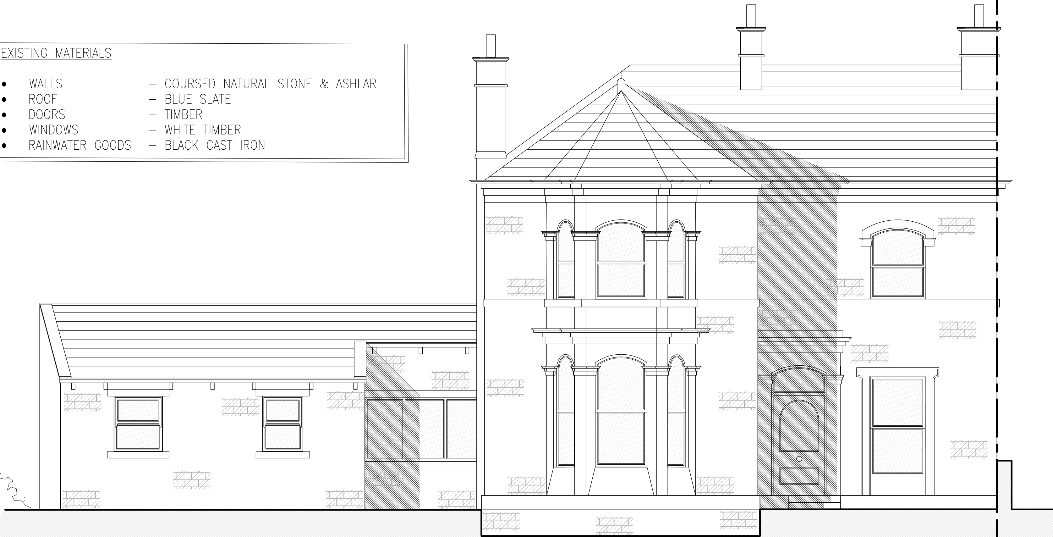
Existing South East Facing Front Elevation Scale 1:50
