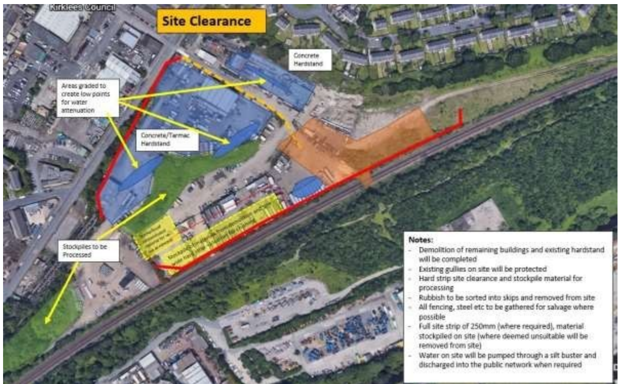
Insert 3-2 Drainage arrangements during site clearance works
