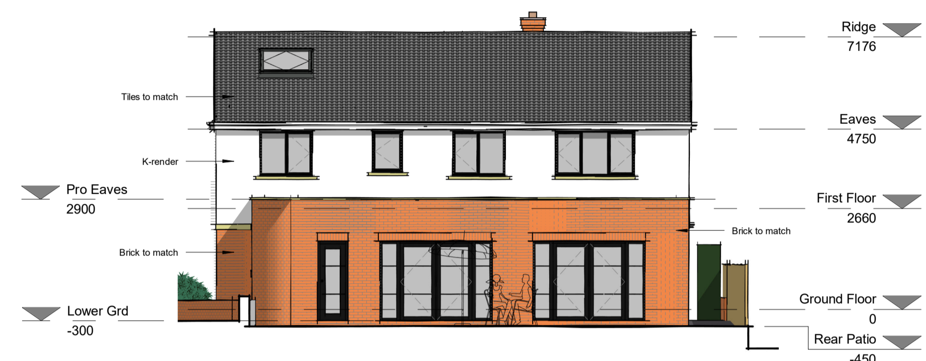
Rear Elevation (West Facing) 1 : 100
