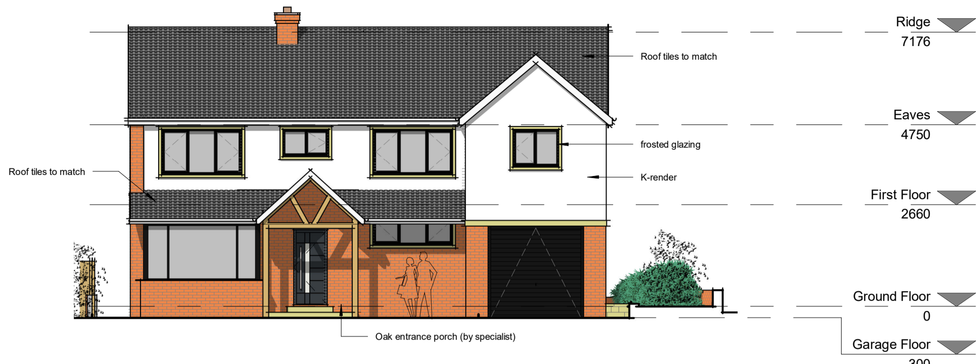
Front Elevation (East Facing) 1 : 100
