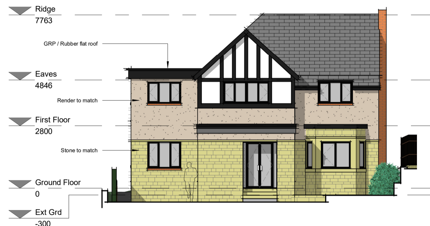
Front Elevation (NW Facing) 1 : 100
