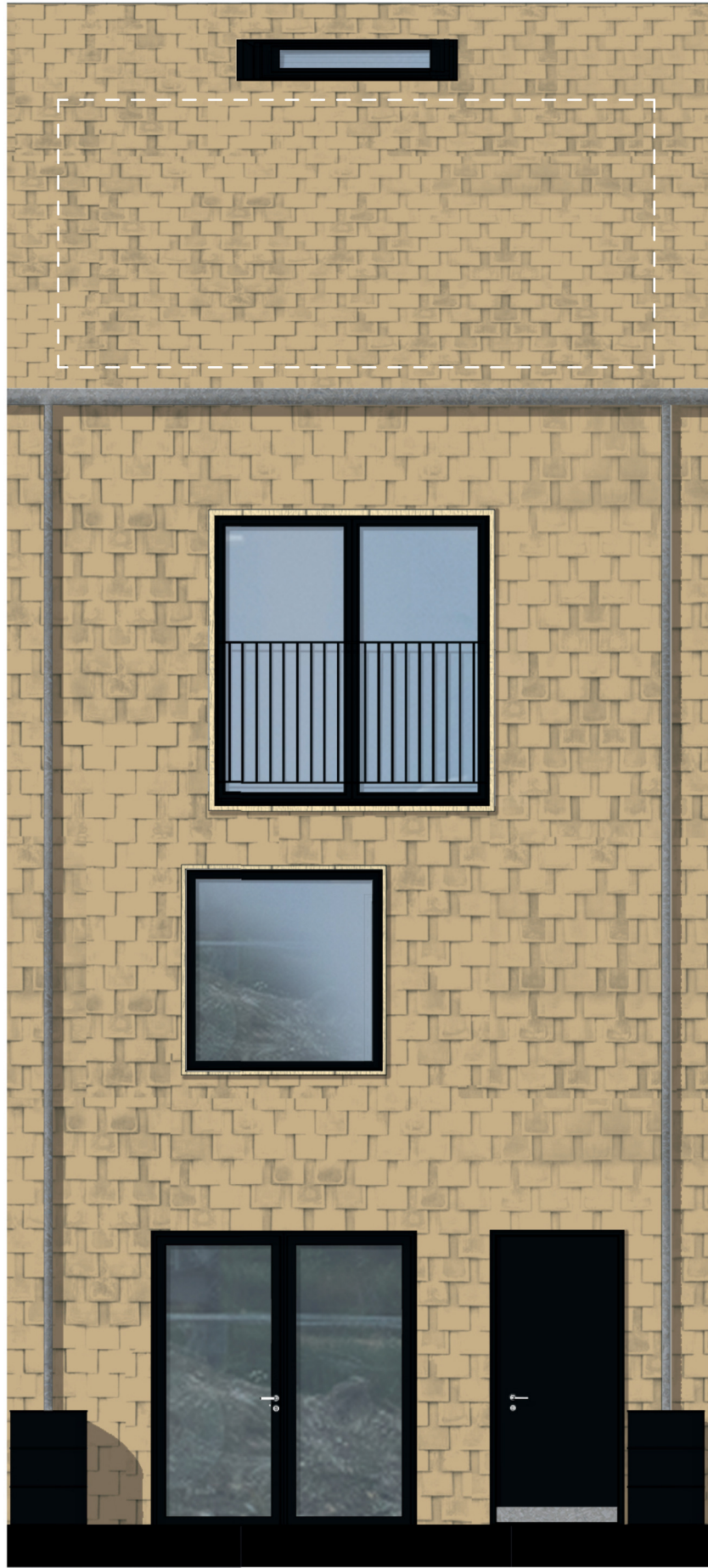
stone slate tile cladding
