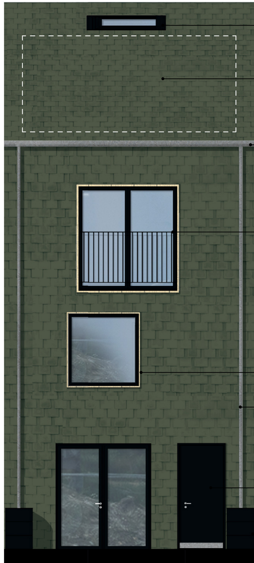
green slate tile cladding
