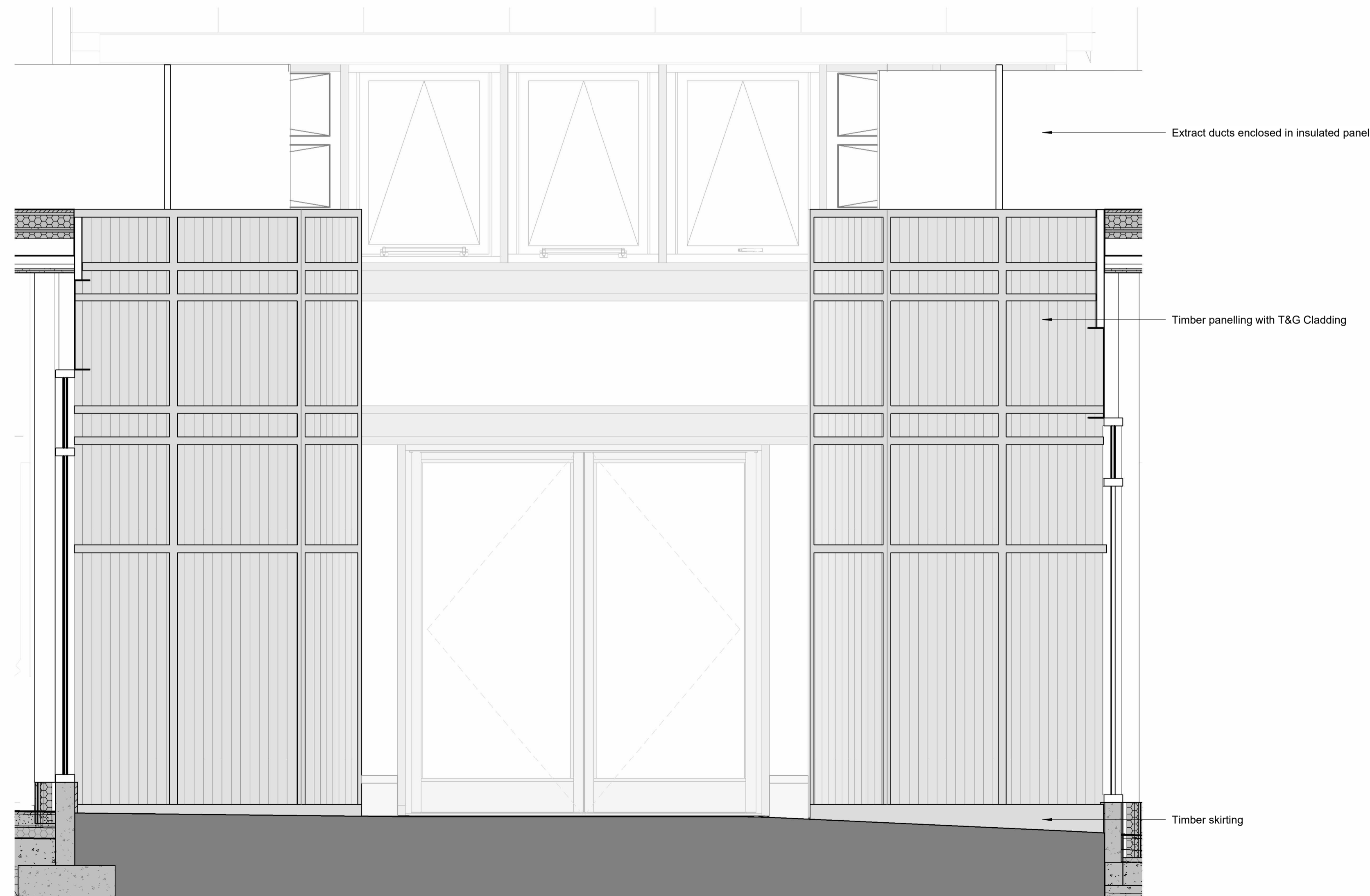
1 ASHP Enclosure Internal Elevation 1:5
