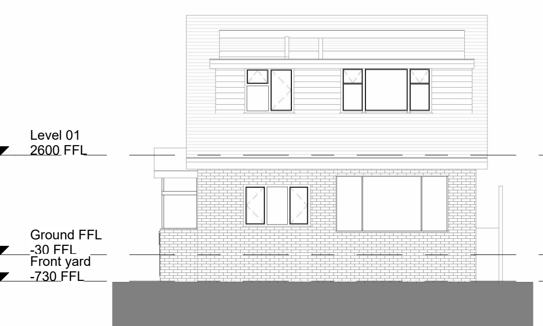
Proposed Front Elevation Scale: 1 : 100
