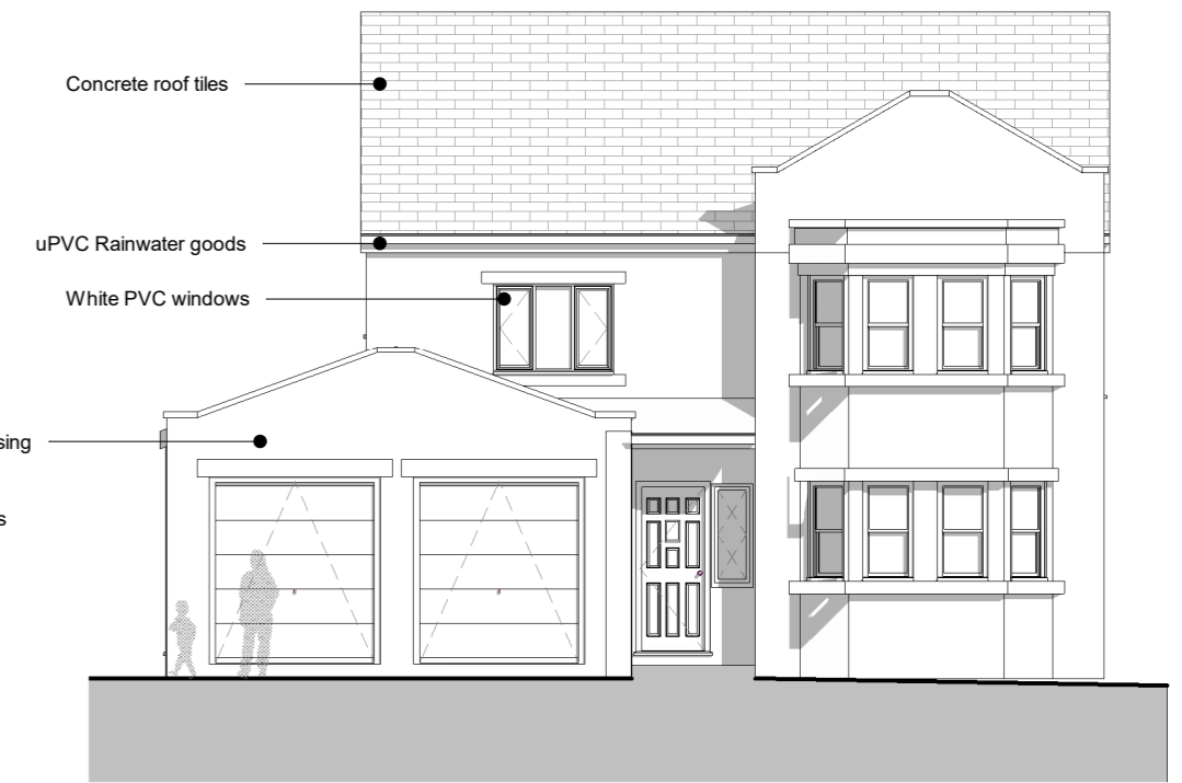
E4 Existing South Elevation 1 : 100
