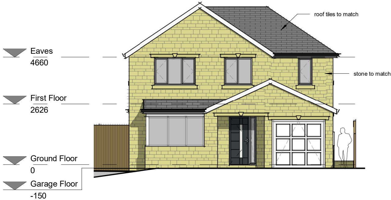
Front Elevation (North Facing) 1 : 100
