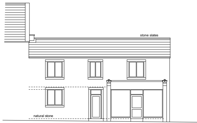
Existing front elevation (1:200)
