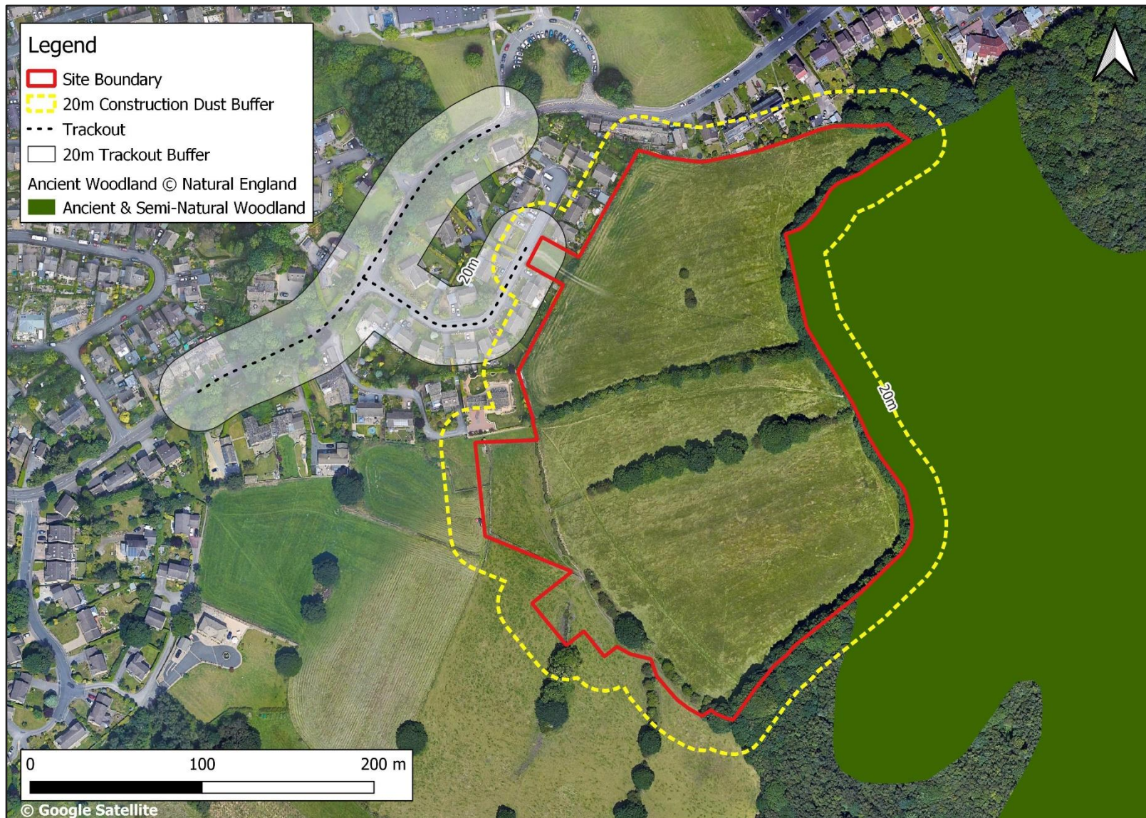
Figure 5-1: Construction Dust Buffers
