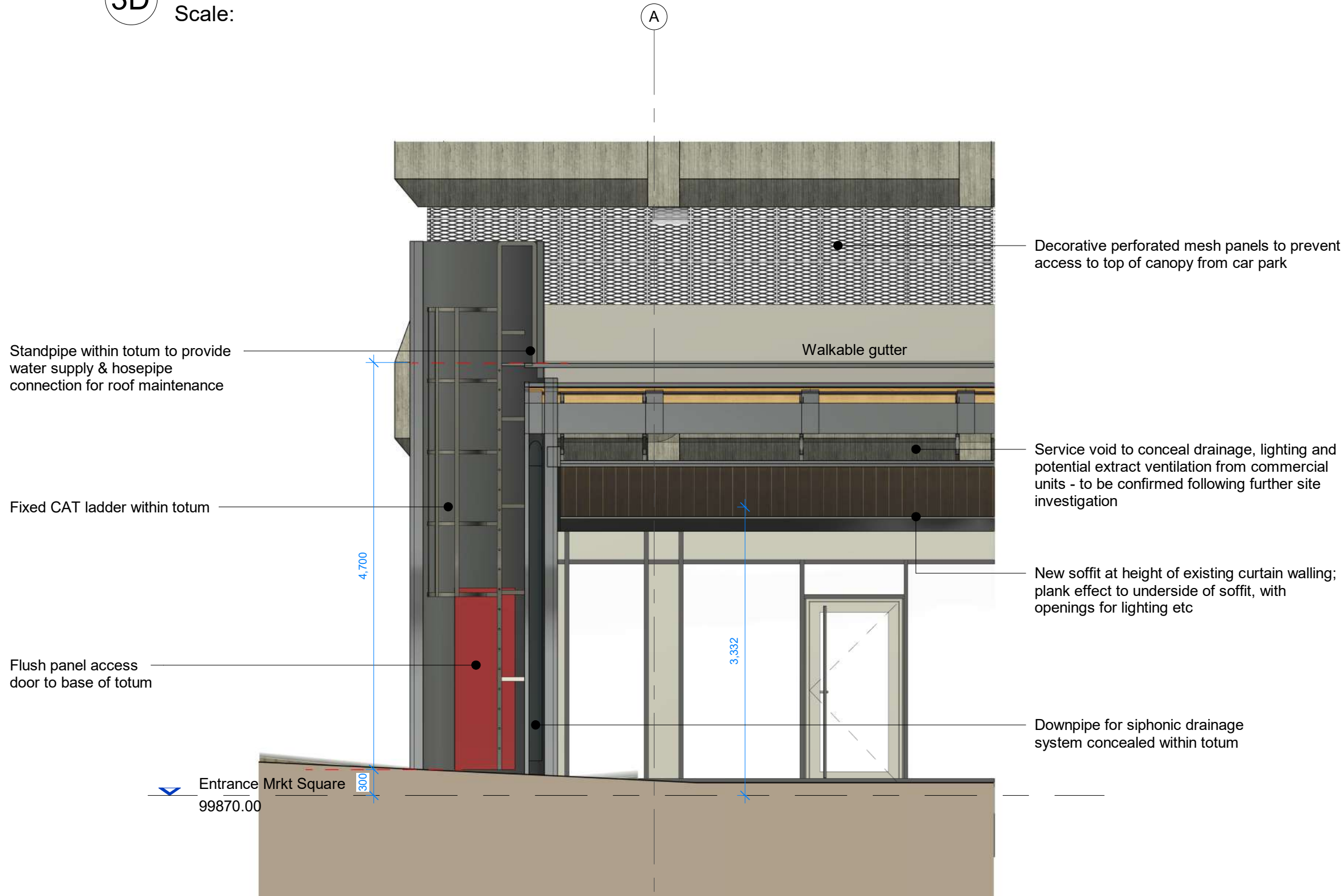
S1 Proposed Totum Section Scale: 1 : 50
