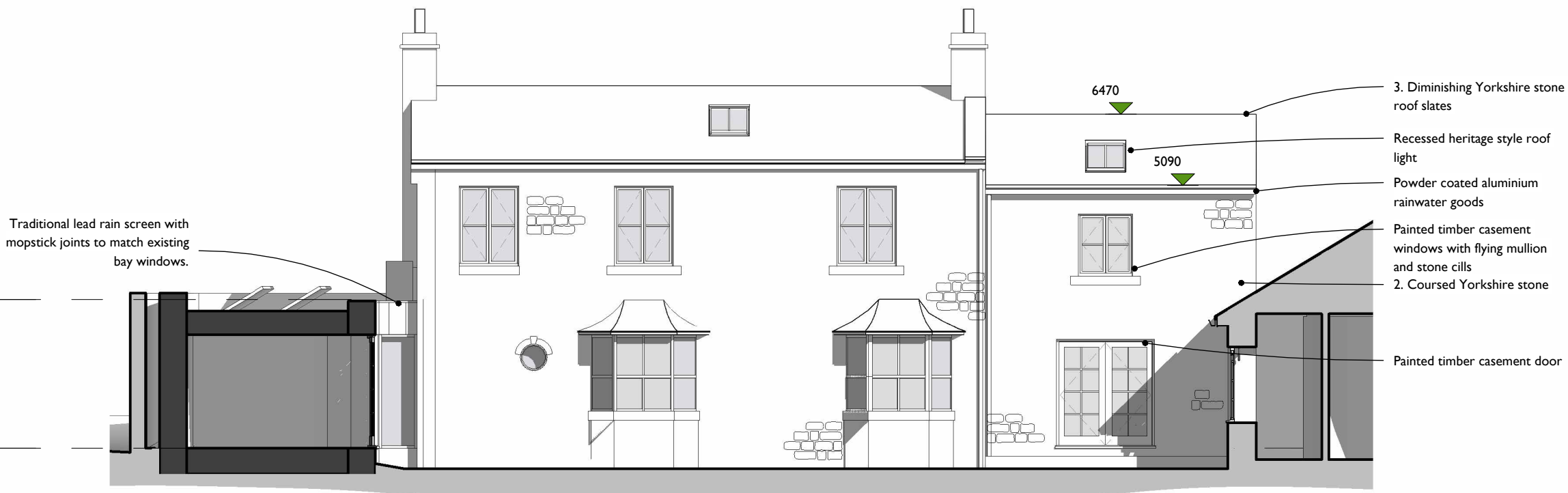
Proposed East Elevation 1 : 100
