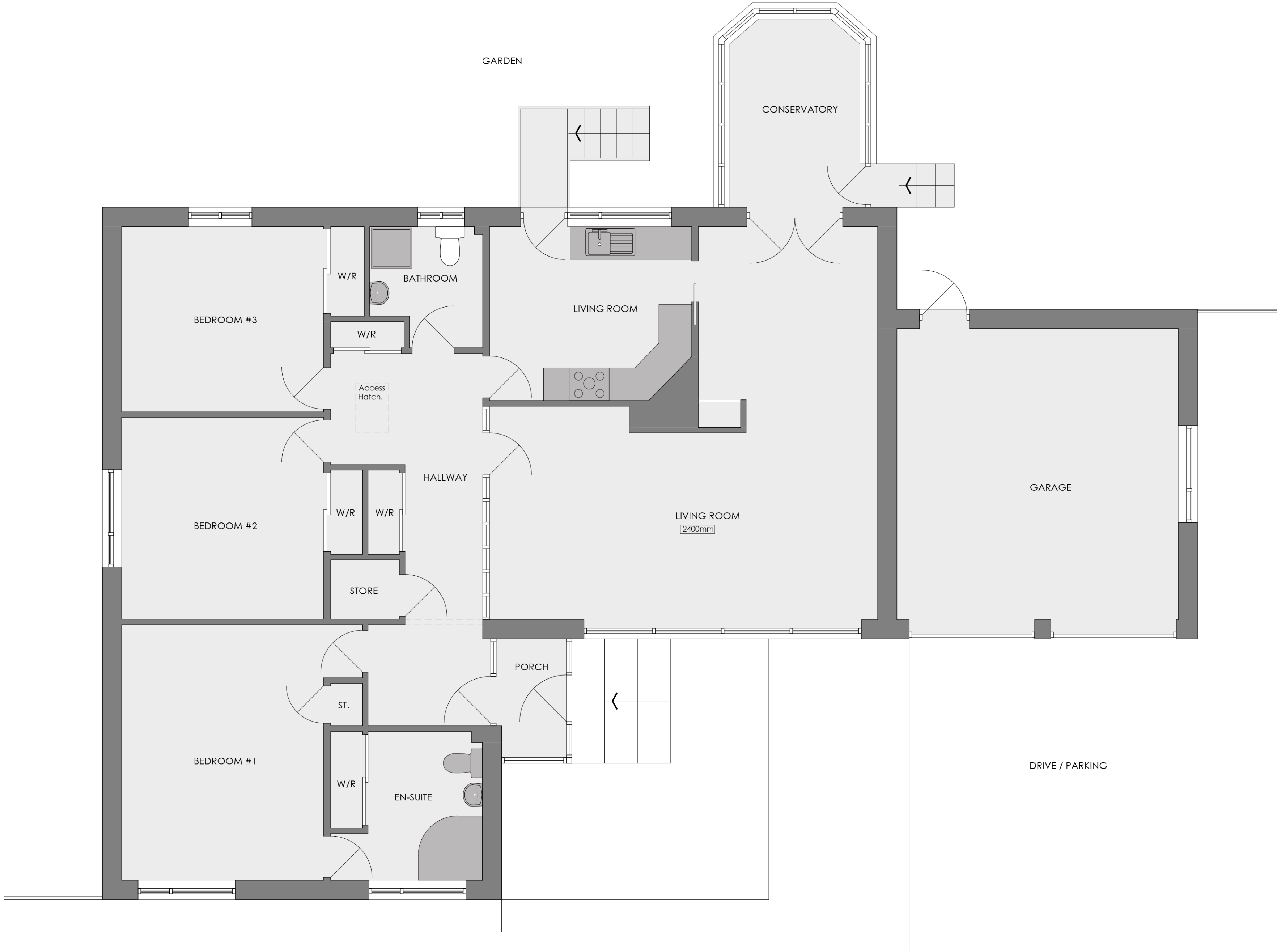
GROUND FLOOR PLAN_ AS EXISTING Scale 1:50
