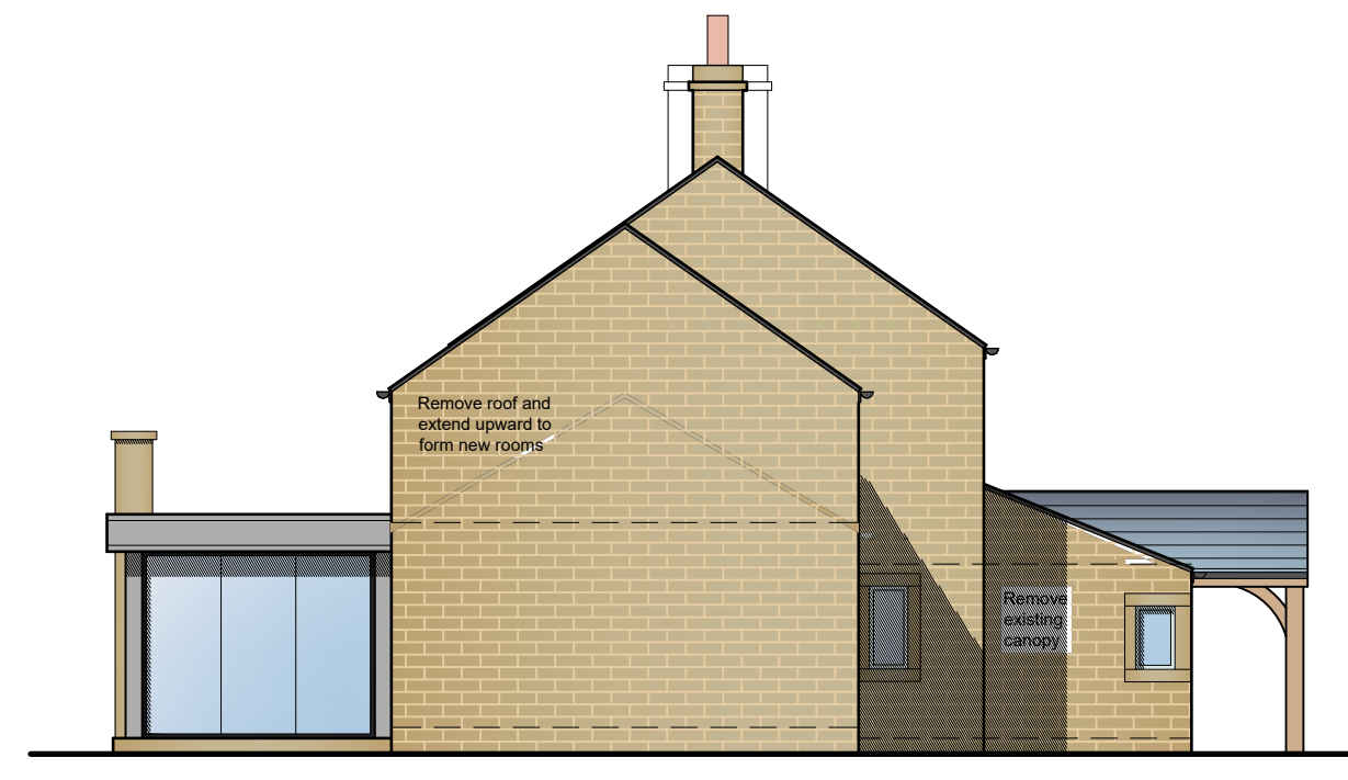
EAST FACING ELEVATION
