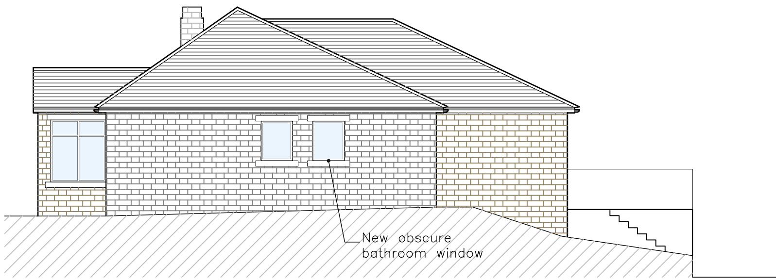
HOUSE SIDE ELEVATION (NORTH)
