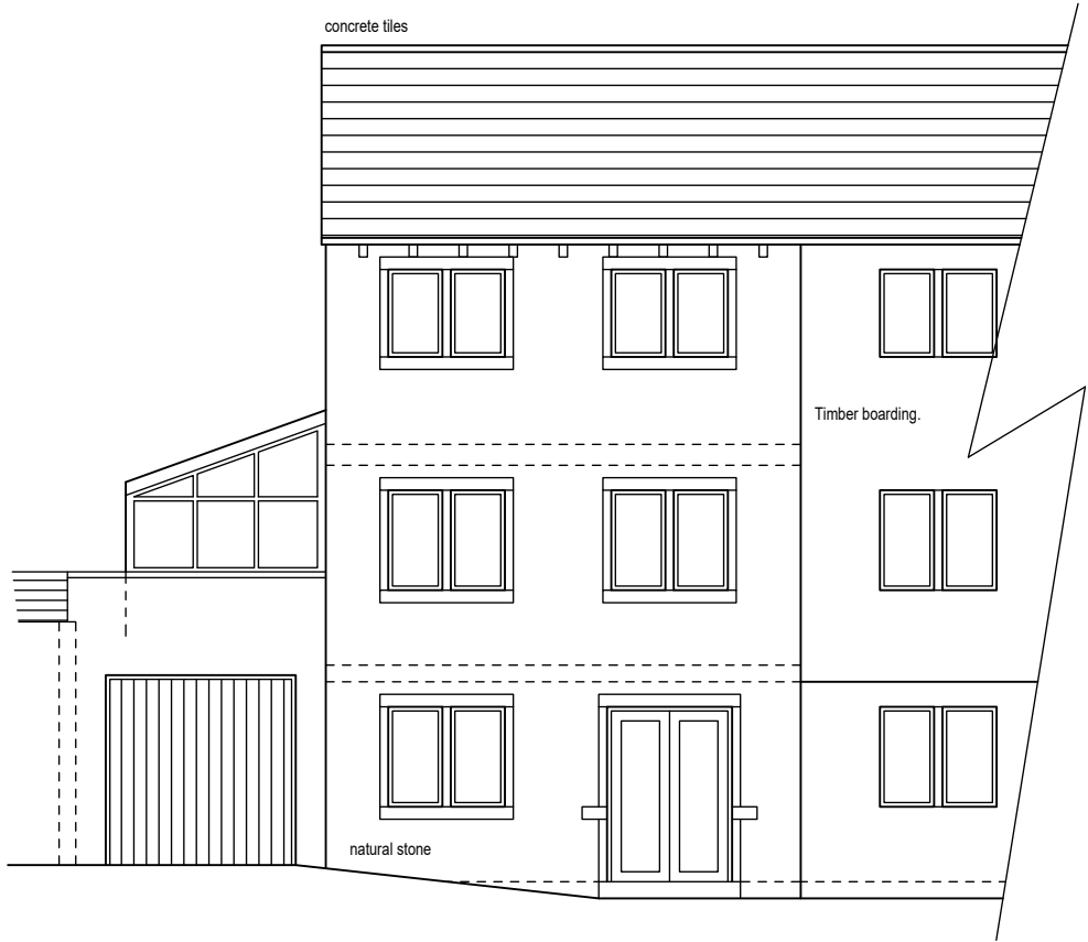
Existing rear/south east facing elevation (1:100)
