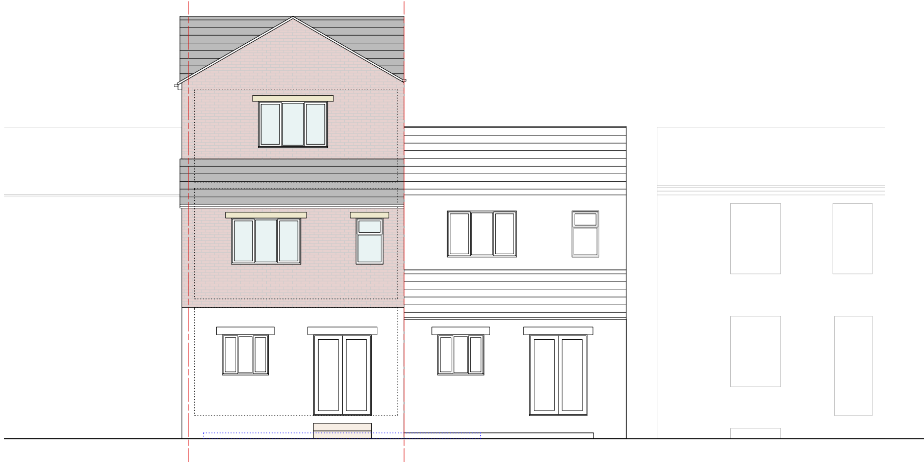
Rear Elevation As Proposed Scale 1:100
